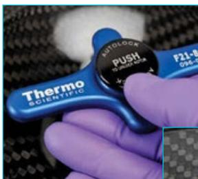
Auto-Lock is identified on Thermo Scientific superspeed centrifuges with a **black push button** and on Thermo Scientific general purpose and small benchtop centrifuges with a **green push button**.
