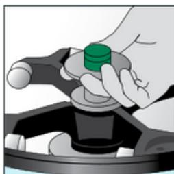
Push center button to remove rotor
