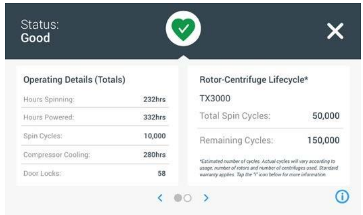
Figure 4: Centrifuge Health Alert Status Icon gives clear indication of a non-dangerous situation and provides recommendations.
