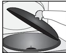
Lift windshielde rotor lid to remove.
