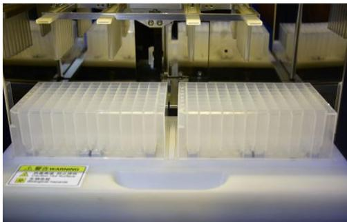
Open the door, pull the tray outward, and remove the seal from the 96-well plate with reagents. Place the notch outwards in the groove of the tray, then push the tray into the compartment; then push the stirring sleeve into the magnetic rod sleeve.
