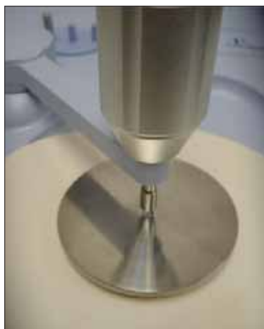
Figure 1. Close-up view of pressure arm and uATR crystal with conical shoe and adaptor.
