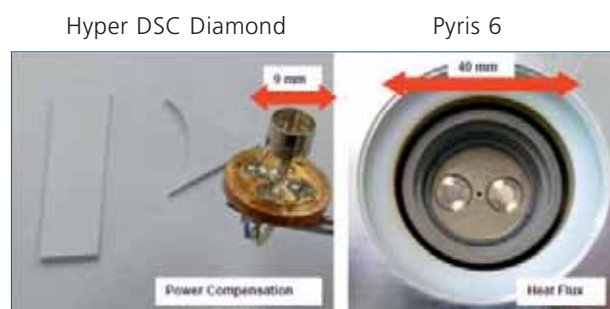
Figure 1. Furnace of HyperDSC versus heat flux DSC furnace.
