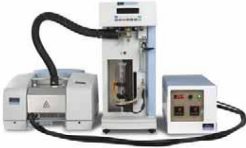
Figure 1. The TL 8000 transfer line couples a Spectrum 100 FT-IR to a Pyris 1 TGA.
