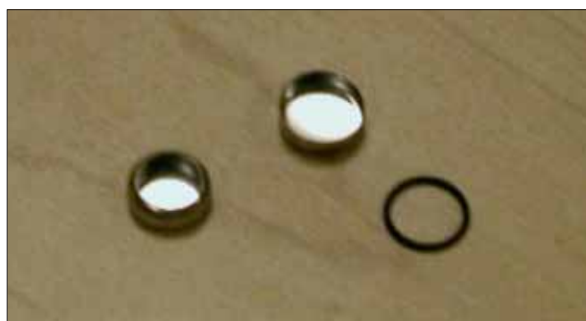
Figure 2. Stainless steel pan (Part Number 03190218) used for this experiment.
